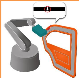
weld seam inspection
